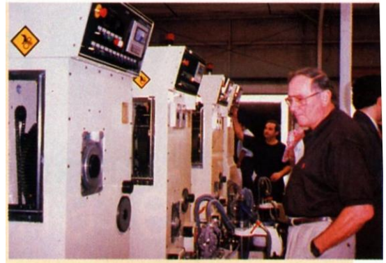
Dick Sharfstein of Pride Container inspects the Tecasa 66-by-141-inch two-color flexo folder-gluer at Central Florida Box Corp.
