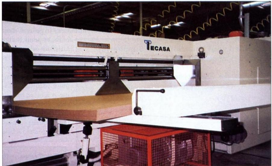
*Above: Central Florida's Merigraph plate making system. Below: The plant's new 66-in. x 144-in. Tecasa two-color flexo folder Bluer.*
